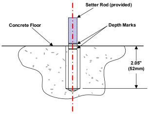
6. Insert four (4) drop-in concrete expansion anchors into drilled holes.
